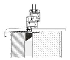
to be provided as insulation, but not for load transfer. Either a knife or scissors can be used for cutting the sealing tape to size.
