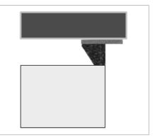
In its final position the sealing strip must not project beyond the edge of the masonry and should be positioned at least 3 mm behind the sealing surface. The sealing surface should be a smooth, level, continuous surface. The processing guidelines for joint sealing tapes apply (see "Fitting the window system" below). Projecting material can be shortened using a knife or scissors.
