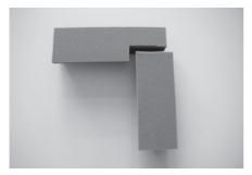
ISO-BLOCO FILLER pieces can be butt jointed to extend their length. For an airtight joint cut the rigid bar back by 2 mm to achieve a defined pressure joint between the impregnated tape sealing strips.
