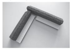
For an airtight seal at the corners, the rigid bar of the vertical profile should be cut back by 2 mm to achieve a defined pressure joint between the 2 impregnated tape sealing strips.
