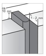
4.As the tape is installed it will expand to fill the joint (time dependant on temperature) making it self supporting. Any gentle unevenness along the joint will be accommodated for by the tape expanding into these areas.
