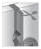
2.Peal back about 10-20 cm of the release paper to expose the self adhesive side of the foam tape.
