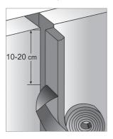
When installing the tape into the joint fix the self adhesive side to the smoothest surface (e.g. window frame) using a trowel, pallet knife or similar flat blade tool. Take care **not** to stretch the tape.
